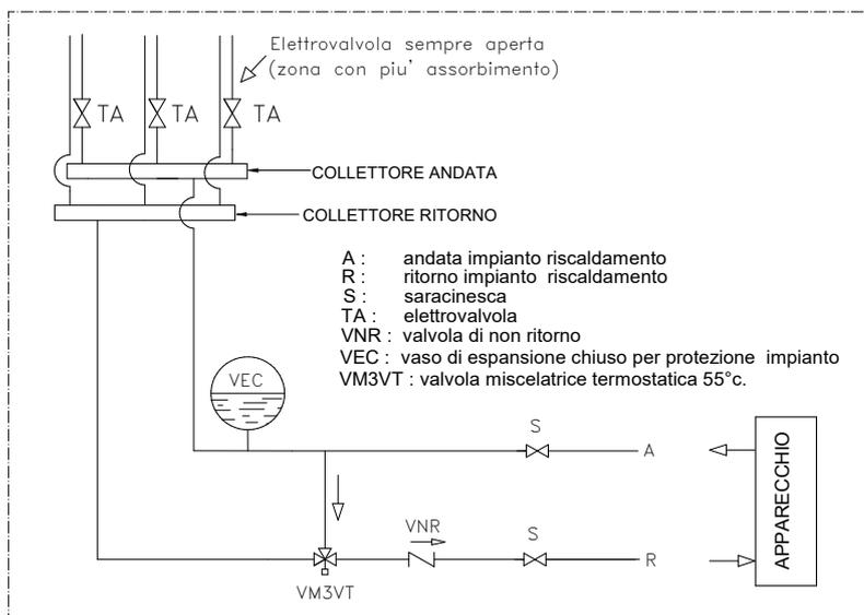
**COMPACT S26 – S32 GT5****5.3 SCHEMA IDRAULICO CON SOLO RISCALDAMENTO**
