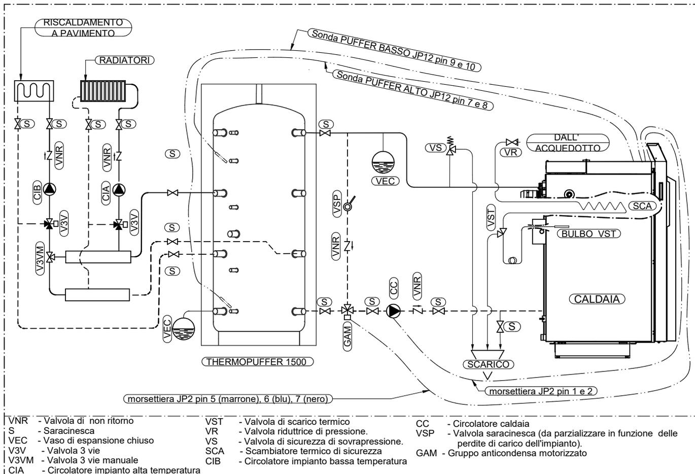
PUFFER 1500 l + CALDAIA + IMPIANTO ALTA TEMPERATURA + IMPIANTO BASSA TEMPERATURA
