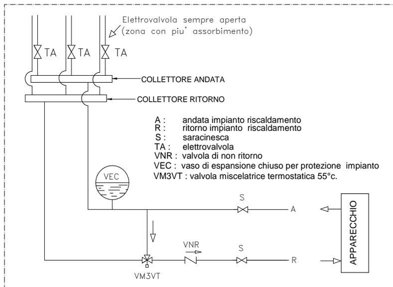
**5.3 SCHEMA IDRAULICO CON SOLO RISCALDAMENTO**
